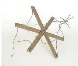
A remnant of the antenna from the first amateur station to work across the Atlantic: A six-wire spreader from a cage antenna used at 1MO-1XW in 1922 and 1923 for the first transatlantic tests. This was donated to the ARRL by K.B Warner, W1EH. [ARRL Photos]
